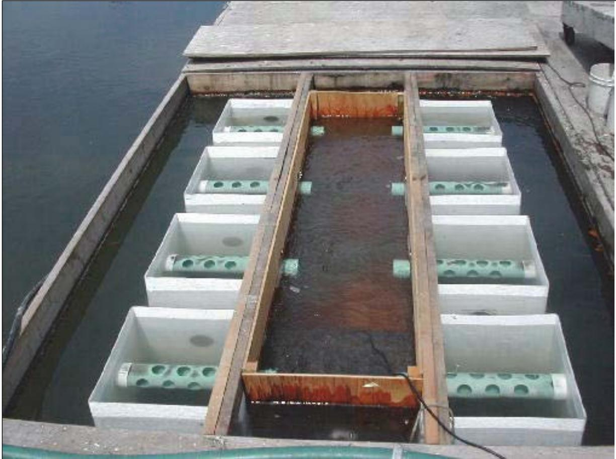
Figure 2. A Floating Upwelling System, or FLUPSY.
